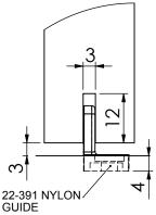
GUIDE SETUP FOR GROOVED DOOR
