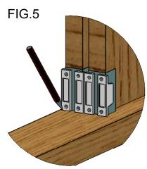
To obtain clearance for guiding, wrap thin cardboard (0.5 - 1.0mm thick) round the edge of each door in turn and mark position of guides when door hangs plumb. See fig.5
