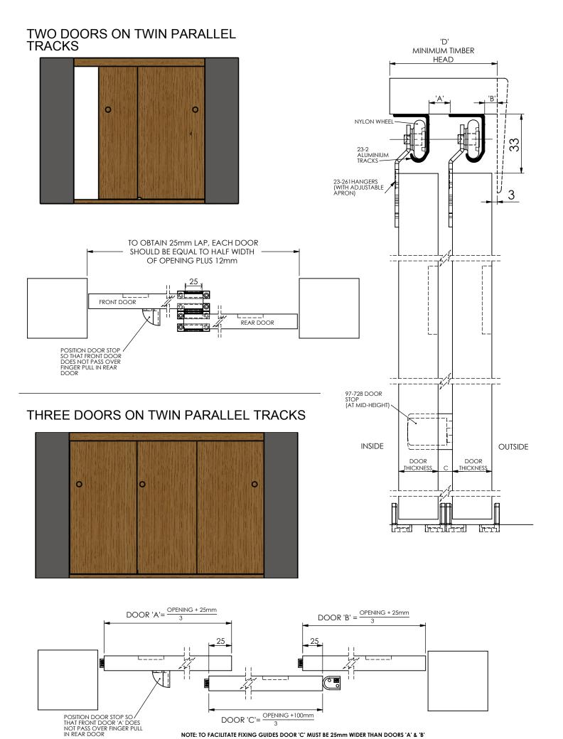
NOTE: TO FACILITATE FIXING GUIDES DOOR 'C' MUST BE 25mm WIDER THAN DOORS 'A' & 'B'
