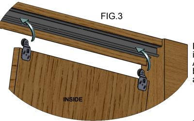
Holding the door at an angle hook the inside door onto the track . See fig.3. Avoid the use of force as hangers may be damaged and the smooth running action impaired.
