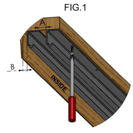
Cut track to required length and fix with No.6 x 20(3/4")woodscrews to soffit/support allowing gaps (Dim. 'B') as shown in fig. 1
