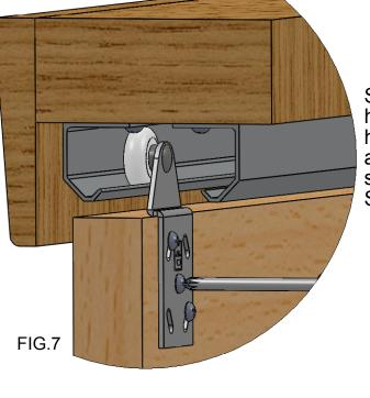
Slightly loosen the two screws in each hanger and adjust doors until they hang plumb and close squarely against the frame. Screw in centre screw to prevent further movement. See fig.7
