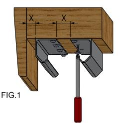
Fix tracks with No.10 x 19(3/4") woodscrews to soffit/support allowing gaps (Dim. 'X') as shown in fig. 1
