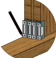
To obtain clearance for guiding, wrap thin cardboard (0.5 - 1.0mm thick) a round the edge of each door in turn and mark position of guides when door hangs plumb. See fig.5
