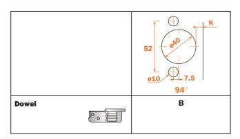
Use this table to identify the available drillings and fixings. Fill the third position of the hinge code number with the letter or the number corresponding to your choice. I.e.: CF\_7A99.
