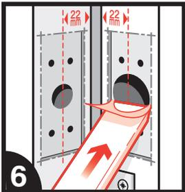
6 Cut out the area required to house the fixing plates on both the door leaf and the door frame.
