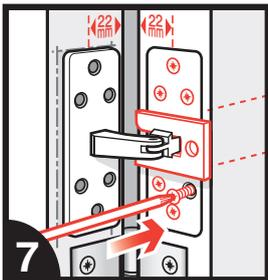
7 Insert the body of the closer into the door leaf, with the retaining plate facing you, and screw fix.
