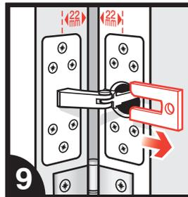
9 Remove the retaining plate. Ensure that it is kept in a safe place in case it is necessary to remove the closer from the door at any time.
