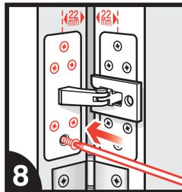
8 Fix the plate onto the door frame making sure it is exactly in line with the other plate.
