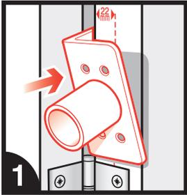
1 Offer up the fitting jig to the door leaf with the lip on the knuckle side of the door just below or above the middle hinge. The centre line should always be 22mm from the knuckle side of the door.
