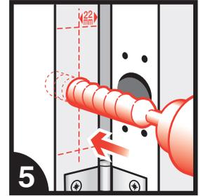
5 Drill out a centre hole 15mm diameter to a depth of 10mm.
