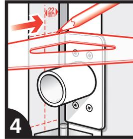
4 Mark the top and bottom edges level and square across to the door frame. Mark a centre line 22mm from the knuckle side of the frame.
