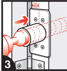
3 Drill the hole for the closer body using the Lewis auger bit.
