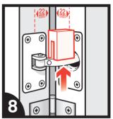
Remove the retaining block. Ensure that it is kept in a safe place in case it is necessary to remove the closer from the door at any time.
