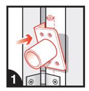
Offer up the fitting jig to the door leaf with the lip on the knuckle side of the door just below or above the middle hinge. The centre line should always be 22mm from the knuckle side of the door.
