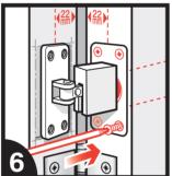
Insert the body of the closer into the door leaf, with the retaining block facing you, and screw fix.
