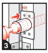
Drill the hole for the closer body using a Lewis auger bit.
