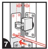
Fix the plate onto the door frame making sure it is exactly in line with the other plate.
