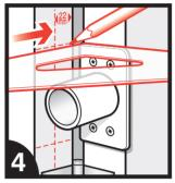
Mark the top and bottom edges level and square across to the door frame. Mark a centre line 22mm from the knuckle side of the frame.
