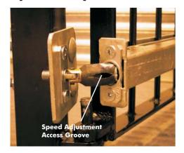
Each ADAPT-A-GATE kit includes an RTS gate closer. The closer is fixed on the gate with a chassis, and a bracket fixes to the gatepost. Joining the closer and the bracket is an articulated joint. When the gate is opened, the articulated joint fixed to the gatepost bracket creates tension in the gate closer's internal spring. When the gate is allowed to close, the closer's hydraulic damping unit provides variable closing speeds to suit.
