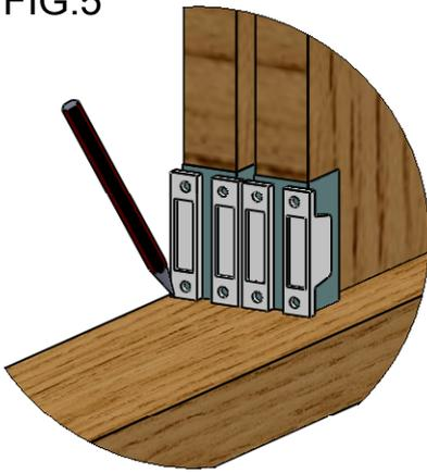
To obtain clearance for guiding, wrap thin cardboard (0.5 - 1.0mm thick) round the edge of each door in turn and mark position of guides when door hangs plumb. See fig.5
