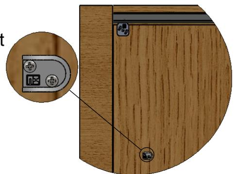
Screw door stop to inside of front door at mid-height with No.6 x 16(5/8") woodscrews. See fig.8.
