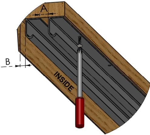
Cut track to required length and fix with No.6 x 20(3/4") woodscrews to soffit/support allowing gaps (Dim. 'B') as shown in fig. 1
