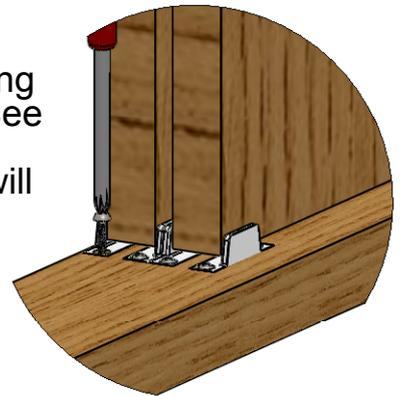
Screw guides down centrally in opening using No.6 x 16 (5/8") woodscrews. See fig.6.
