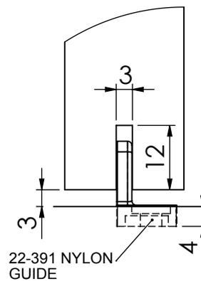
GUIDE SETUP FOR GROOVED DOOR
