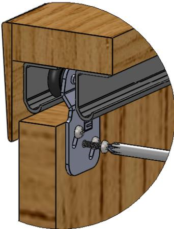
Ensure that door hangs plumb with frame, adjust by using slotted holes, then put in centre screw to prevent further movement. See fig.7
