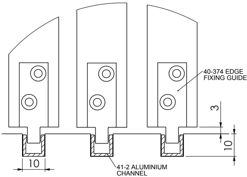
ALTERNATIVE GUIDE USING ALUMINIUM CHANNEL
