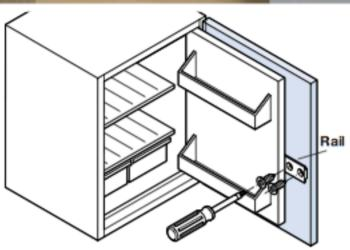
Open the refrigerator door by 90° and insert the rail into the guide (see "X" on plan drawing). Screw on the rail exactly horizontally on the inner side
